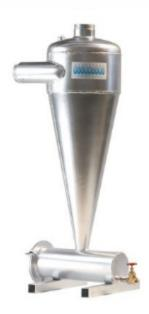
It can separate water from sand. It is made of hot galvanized steel, cone-shapped. The flow entrance is tangential to the cylindrical part, so that, the flow which is linear at the beginning, is changed into an angular flow, which practises a centrifugal force.
