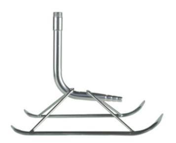
It is particularly suitable for low pressure sprinklers, under - foliage irrigations, meadows, where it can be easily moved, thanks to its two lateral shoes. It is entirely made of hot galvanized steel. It is supplied with the upper joint Ø  $^3$ 4" - 1" male or female, and the lower point has been studied for plastic pipe, or threaded for fast connections.
